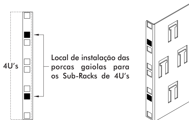
Sub-Racks com 4U's de altura
